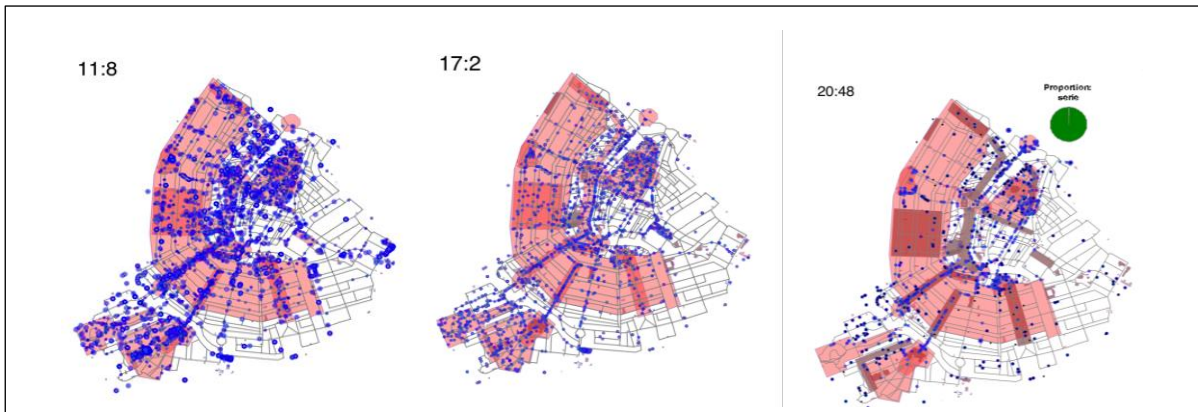
Figure 4.2. Running model. Model destinations (Red = open destinations, color intensity increasing with the number of visits. Grey = closed destinations) and agents (blue dots)
